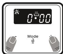
1. Press the "+" and "-" keys simultaneously.
