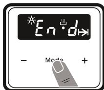
2. Press “MODE” until you see “end” and
