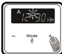
6. Select the desired finishing time using the “+” and “-” keys.
