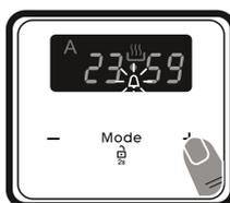
2. Select the desired time period using the "+" and "-" keys while
